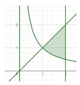
$$\int_{1}^{2} \left[ \int_{1/x}^{x} f(x, y) dy \right] dx$$
