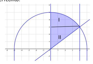
$$\int_0^3 \left[ \int_0^{\frac{4}{3}y} f(x,y) dx \right] dy + \int_3^5 \left[ \int_0^{\sqrt{25-y^2}} f(x,y) dx \right] dy$$
